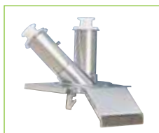
Straight and bias cut hole hopper.
